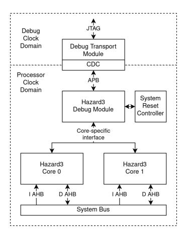
The DM *must* be connected directly to the processors without intervening registers. This implies the DM is in the same clock domain as the processors, so multiple processors on the same DM must share a common clock.
