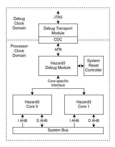
The Debug Module *must* be connected directly to the processors without intervening registers. This implies the Debug Module is in the same clock domain as the processors, so multiple processors on the same Debug Module must share a common clock.
