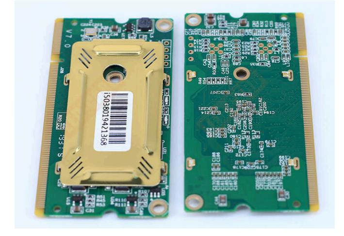
Like other members of the Colorlight family (the Colorlight 5A-75B comes to mind), the i5 is 'real' product that is designed for one specific purpose: it is a controller for large LED video panels. And that's a huge plus, because in FPGA land, high volume means low cost, usually much lower than buying individual components on Digikey or Mouser.
