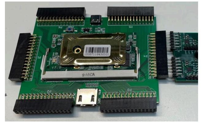
In this case, the center pins can't be used and the number of usable GPIOs per 30-pin connector drops to 16, 8 for each PMOD.
