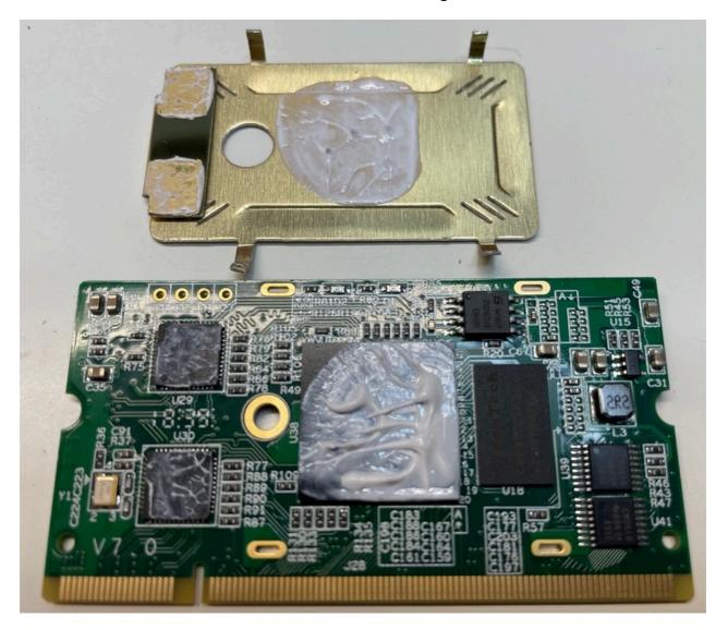
The heat sink is pretty easy to remove without damaging the board.
