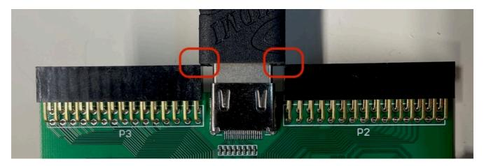
You need a HDMI cable with a narrow connector to make things work, or don't solder connectors P2 and P3, which is what I did.
