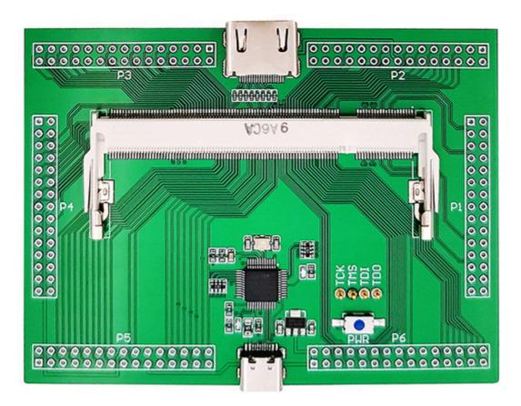
Muse Lab also sells a number of other interesting hobby FPGA boards, such as the ICE40 UP5K based iCESugar, but the ECP5 FPGA on Colorlight i5 has a much larger capacity, so I bought their module + development board combo for \$50 and gave it a try.
