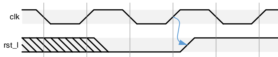
Figure 14-10 Conceptual Clock and Reset Timing Relationship
