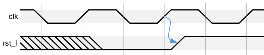
Figure 12-10 Conceptual Clock and Reset Timing Relationship
