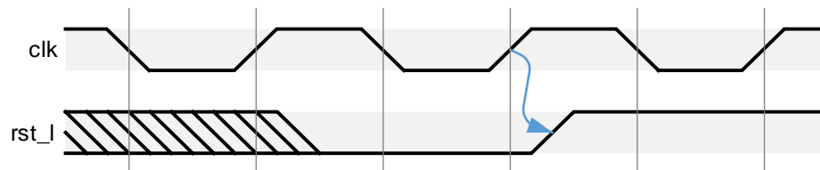
Figure 12-10 Conceptual Clock and Reset Timing Relationship
