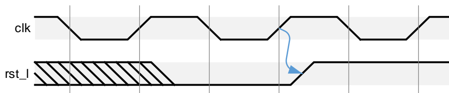
Figure 12-10 Conceptual Clock and Reset Timing Relationship
