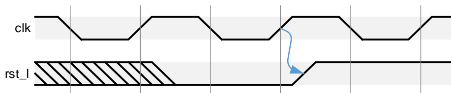
Figure 14-10 Conceptual Clock and Reset Timing Relationship
