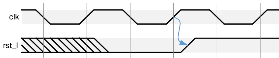
Figure 12-10 Conceptual Clock and Reset Timing Relationship
