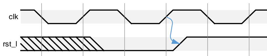
Figure 12-10 Conceptual Clock and Reset Timing Relationship
